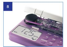
Insert the giving set into the pump and open the clamps on the 2-Pack connector
