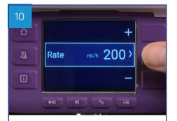
Set rate by pressing the +/- buttons. Press the middle button to confirm
