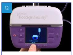
Press and hold the fill set button, after 2 seconds the pump will start
