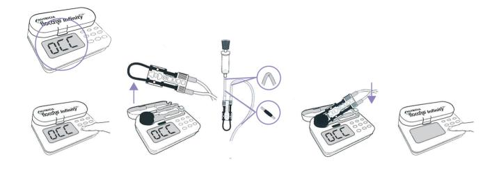
1 5 2 3 4 Press the Start/ Detach the Solve the Re-insert the Press the Start/ Stop button. feeding set. occlusion feeding set. Stop button. problem. (see next page)
